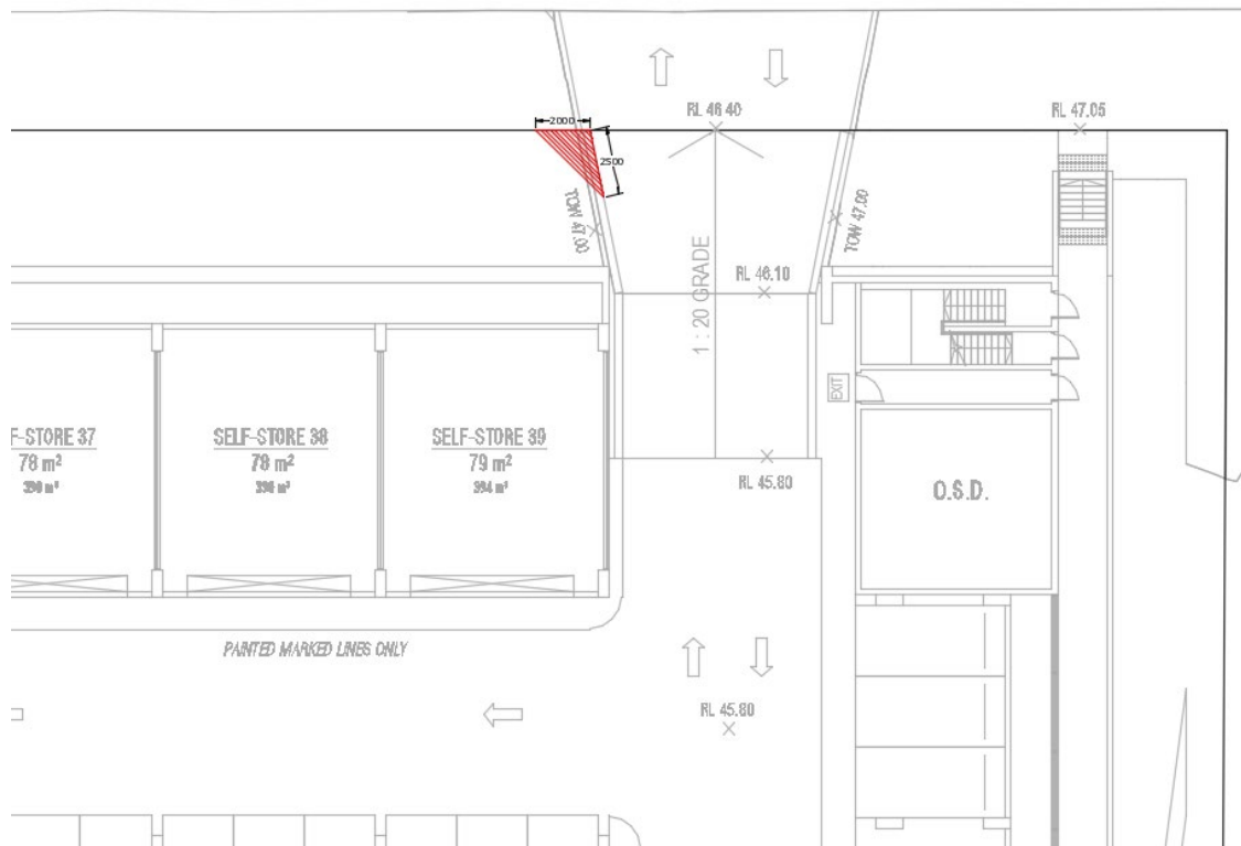
Figure 4-2 Sight Triangle for the driveway in Basement 1
